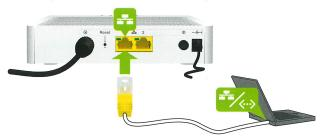
If you want to connect a device using a wired (Ethernet) connection:
